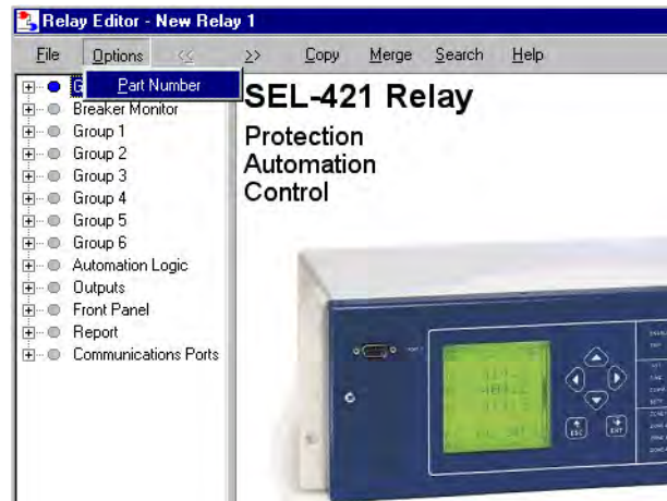
Figure 3.15 Retrieving the Relay Part Number
