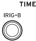
Figure 4.63 TIME BNC Connector, new hardware
