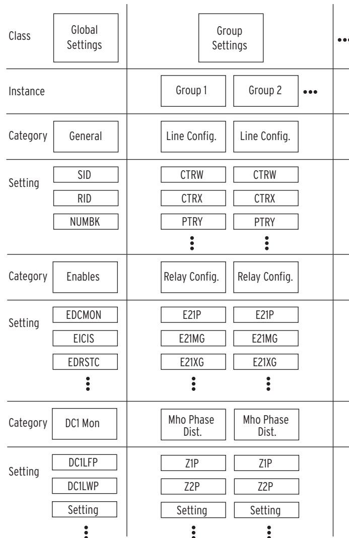
Figure 4.10 Relay Settings Structure Overview
