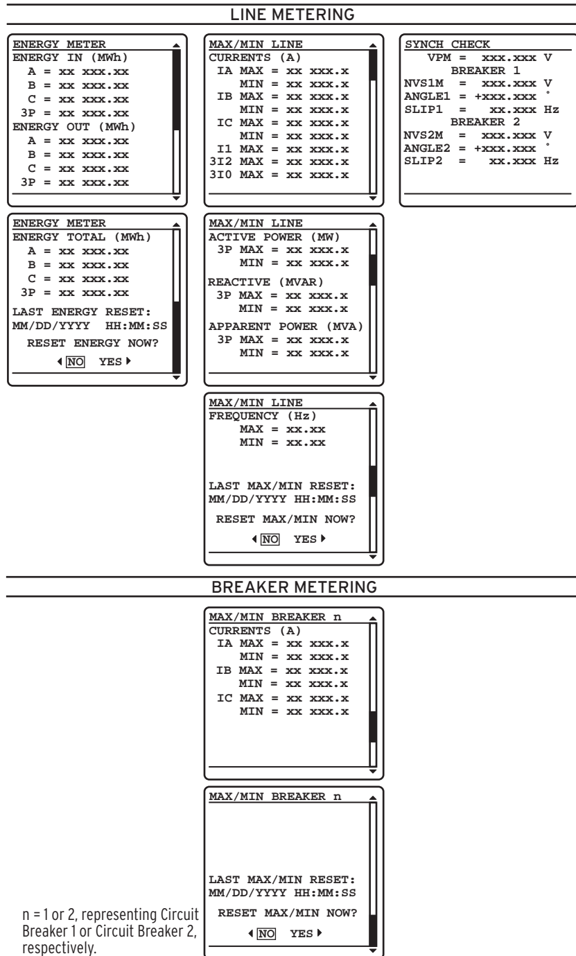
Figure 5.20 ENERGY, MAX/MIN, and SYNCH CHECK Metering Screens
