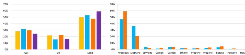
Fig.2 - Rubber pyrolysis yields (left) and gas composition (right)
