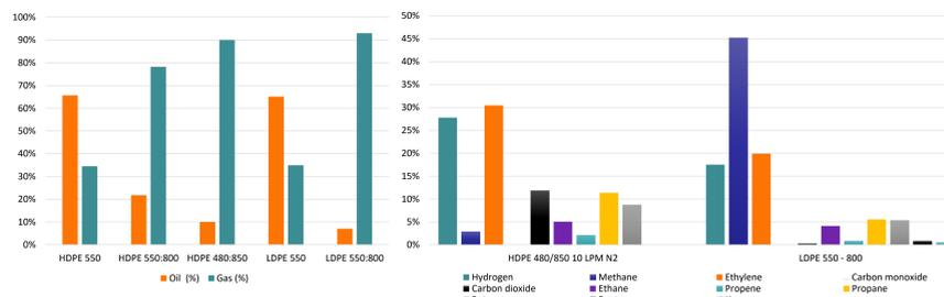
Fig.1 - HDPE and LDPE pyrolysis yield (left) and gas composition (right) for single and double stage configuration
