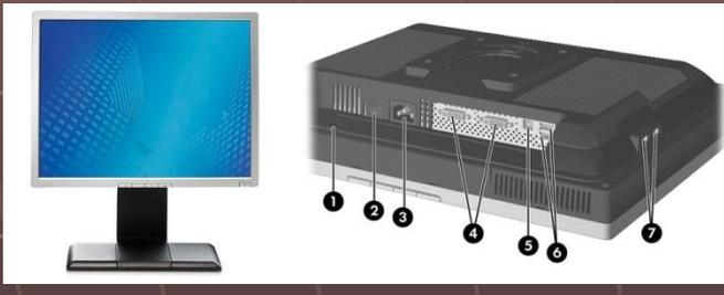
Colour monitor comprising a 20.1 inch (51 cm) TFT LCD (thin film transistor liquid crystal display) active matrix panel combined in the same housing with control circuitry, one USB (Universal Serial Bus) downstream connector, four USB (Universal Serial Bus) upstream connectors, two DVI-I (digital visual interface - integrated digital and analog) connectors and front panel controls (Menu, Minus/Auto, Plus, Input Select, Power).
