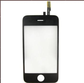
*A touch screen, laminated with tempered cover glass. It is cut in the shape of the front face of a specific mobile phone with two holes, one for the main button and the other for a speaker. It is also equipped with a flexible printed circuit board (FPCB) with a mounted touch integrated circuit (IC). It is used for a specific mobile phone. It has no function of displaying.*
