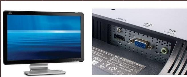
Colour monitor comprising a 23 inch (58.4 cm) TFT LCD (thin film transistor liquid crystal display) active matrix panel combined in the same housing with **integrated speakers, control circuitry, one VGA (Video Graphics Array) connector, one HDMI (High-Definition Multimedia Interface) connector, one Audio-In connector** and front panel controls (Menu, Minus/Volume, Plus/Source, Select/Auto).
