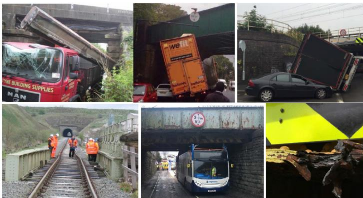
Figure 1 Examples of bridge strikes on the UK rail network. (Source - Network Rail)
