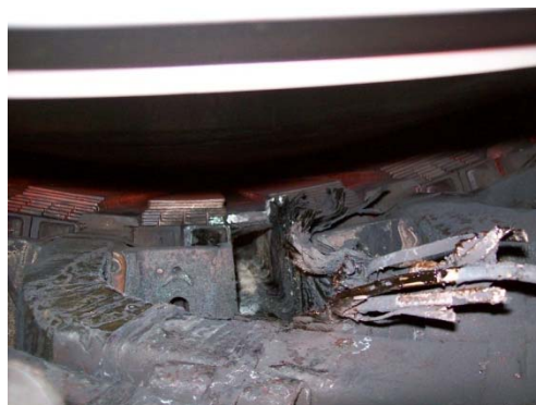
Figure 13A. Winding Damage - Broken Stator Winding Conductor
