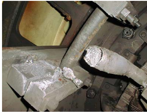
Figure 13C. Burned Away Copper - Fractured Connection Ring
