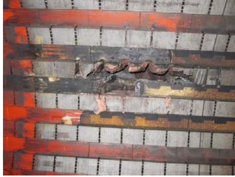
Figure 13B. Core and Winding Damage - Burned Open Bar in a Slot
