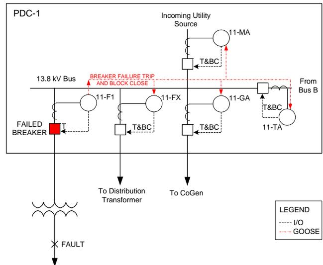
Figure 3. GOOSE eliminated hard-wired breaker failure lockout relays.
