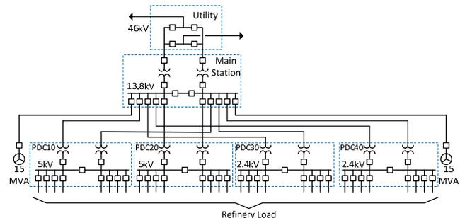
Figure 1. Single line diagram showing new medium voltage infrastructure
