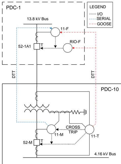
Figure 2. Redundant transfer trip paths employed for transformer protection.
