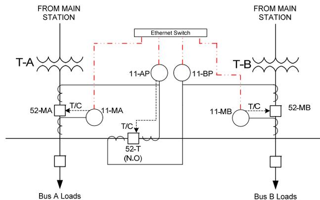
Figure 6. Automatic transfer and manual transfer scheme overview
