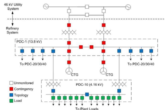
Figure 7. Various breaker types monitored by the load preservation system.
