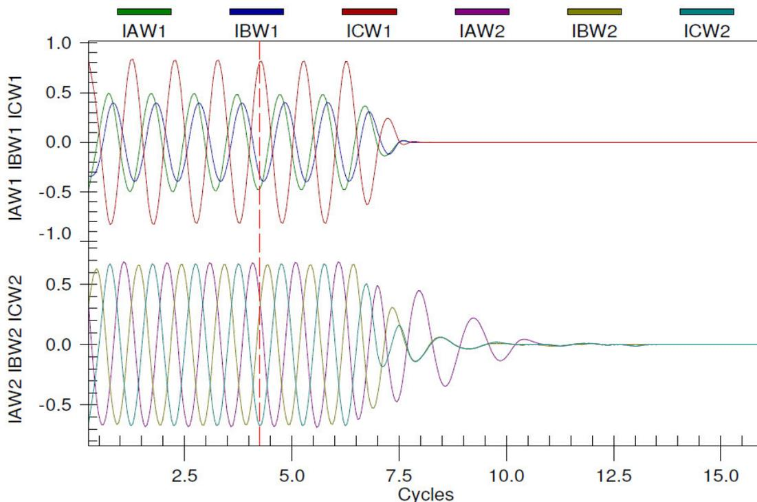
Figure 7 Waveform from a mysterious trip of a Dy1 transformer
