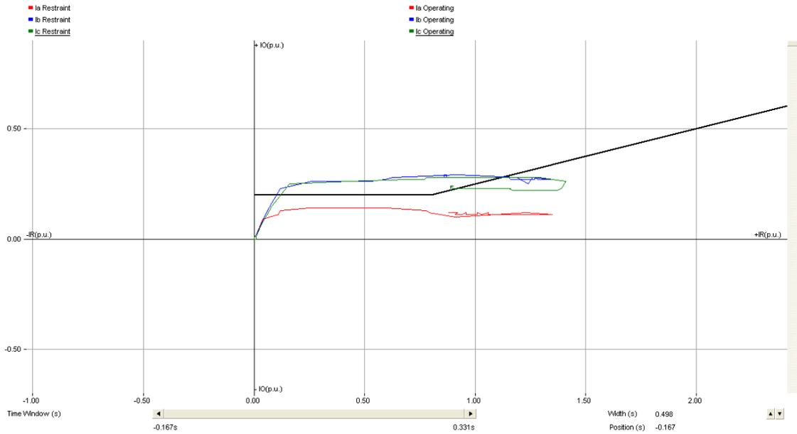
Figure 6: (Iop, IR) indicates differential trip without proper restraint
