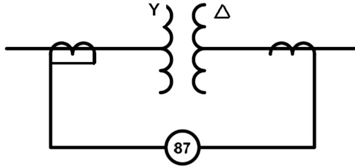
Figure 2 Concept of transformer differential protection
