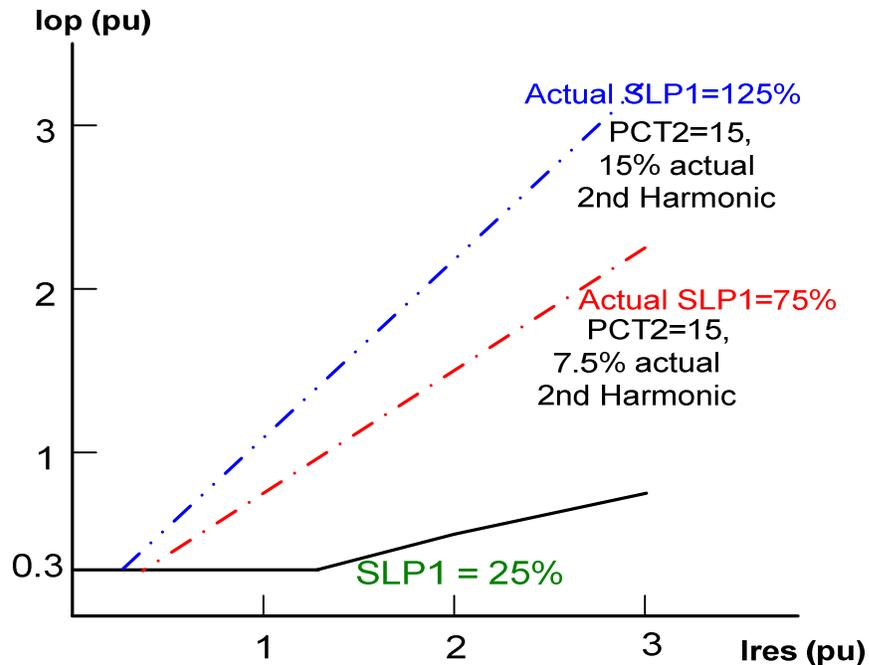
Figure 4. Dynamic shifting of operating curve for harmonic restraint
