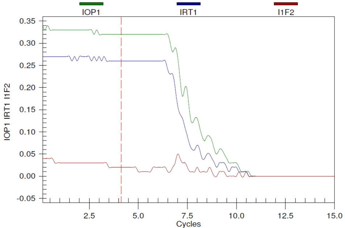
Figure 8 Recorded operating, restraint and 2<sup>nd</sup> harmonic current.
