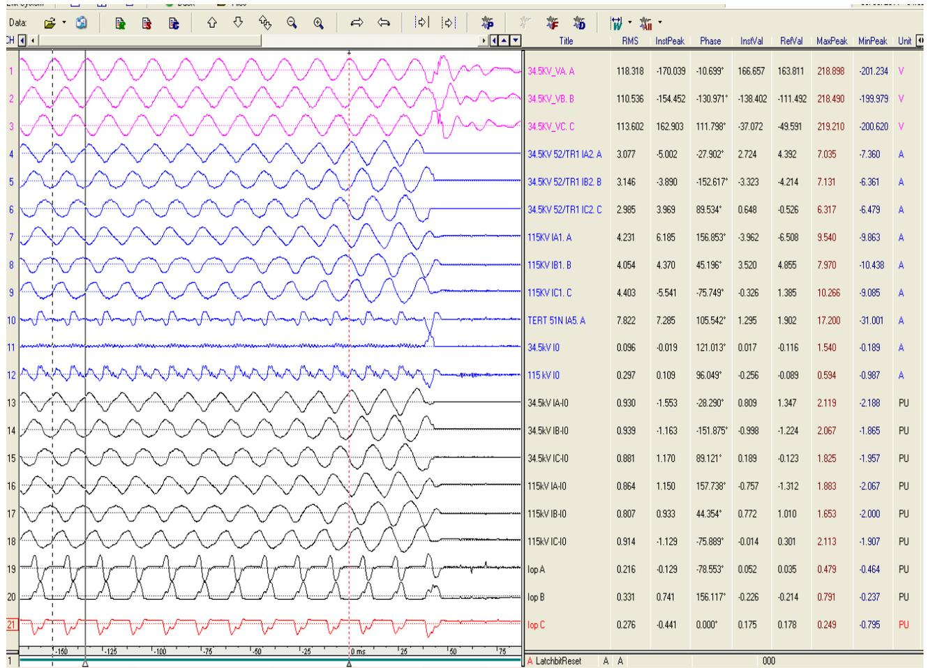
Figure 5: Field recorded waveforms and derived current waveforms for differential study
