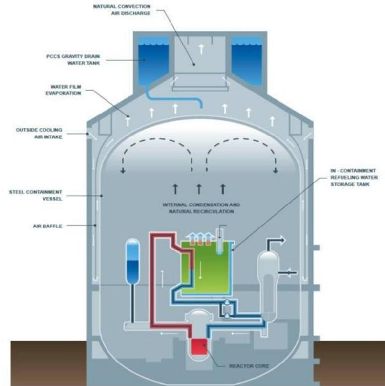
The AP1000 plant is designed to reduce or eliminate the chances of a core meltdown and explosion in situations where the plant experiences a total loss of power, similar to the accident at Fukushima.
