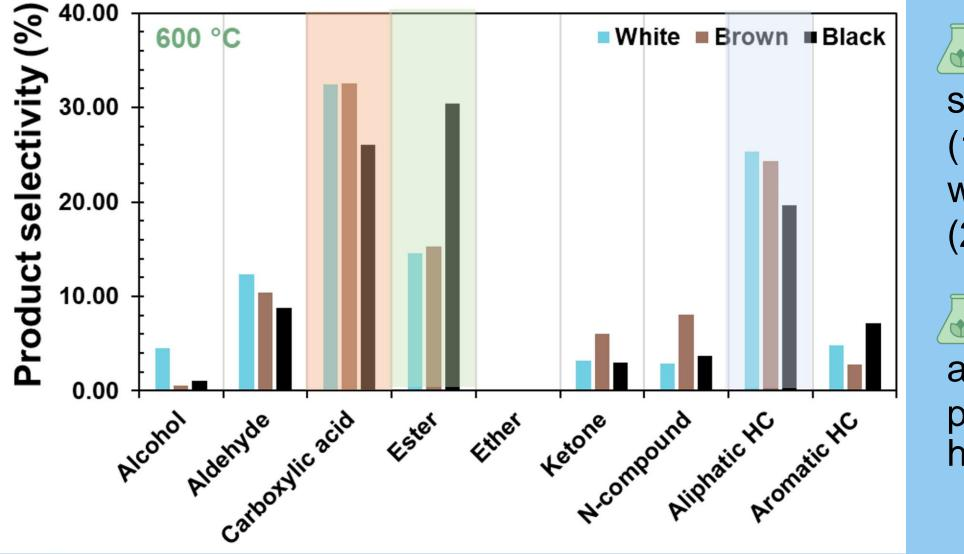
The pyrolysis vapors of white-coated scrap contained a high proportion of ester (14.60%) and carboxylic acid (32.48%) with small amount of aliphatic HC (25.34%) and aromatic HC (4.82%).
