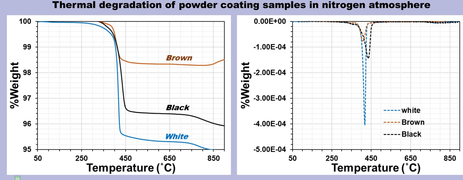
A major thermal degradation of all powder coating samples was occurred at 300-480°C associated to the decomposition of polymeric fraction. The weight loss for the white-coated, black-coated, and brown-coated scrap were 5.03 wt%, 4.08wt% and 1.49 wt%, respectively
