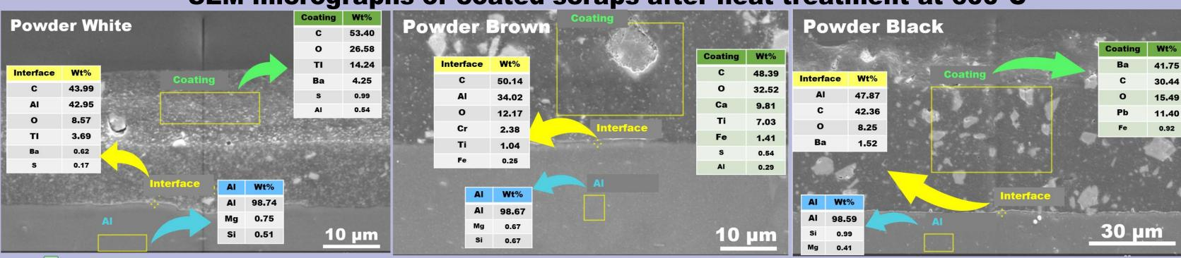
After heat treatment at 600°C, the ash composition was determined by EDX technique. The main compositions of white-ash and brown-ash were C, O, Ti and Ca, while the element of black-ash consisted of Ba, C, O and Pb, respectively. The nonvolatile fraction at the end of heat treatment was chiefly associated to  $TiO_2$ , CaO as the pigment component, and also  $BaSO_4$  as a filler for formulating the pigment for powder coating process.
