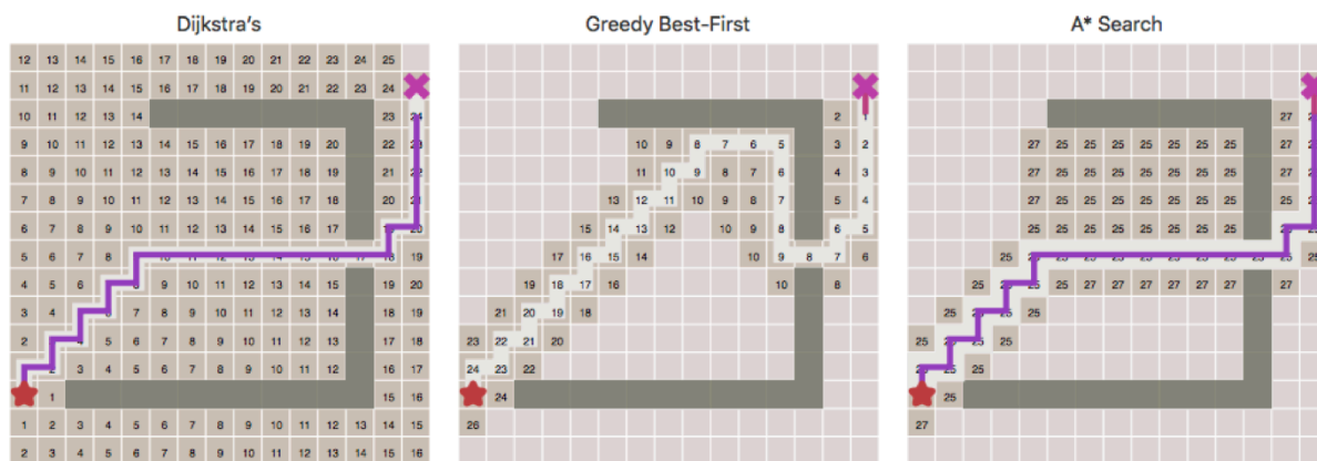
Figure 1. An illustration of classic path planning algorithms in robotics. A* (A-star) remains widely used and provides the optimal path without requiring a global search of the space.
