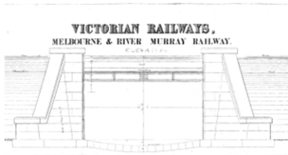
Figure 1 – Historical drawings of Sunbury culvert (L), Existing culvert before widening works (R)
