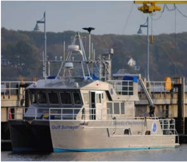
Fig. 8. The R/V Gulf Surveyor , the Center for Coastal and Ocean Mapping's survey platform. The Garmin echosounder is mounted on the port hull, and the Odom on the starboard.
