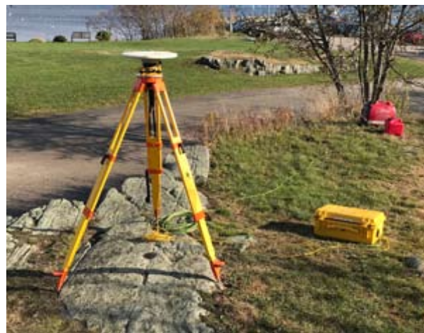
Fig. 7. Trimble geodetic GNSS observation station over NGS horizontal control mark AB2631.
