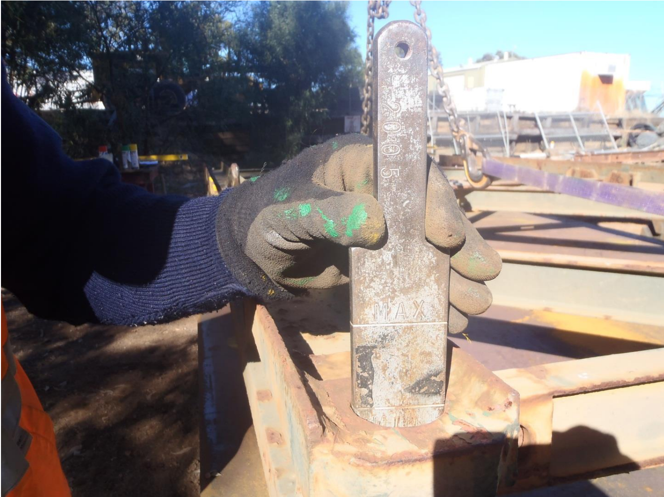
Measuring pin hole wear
