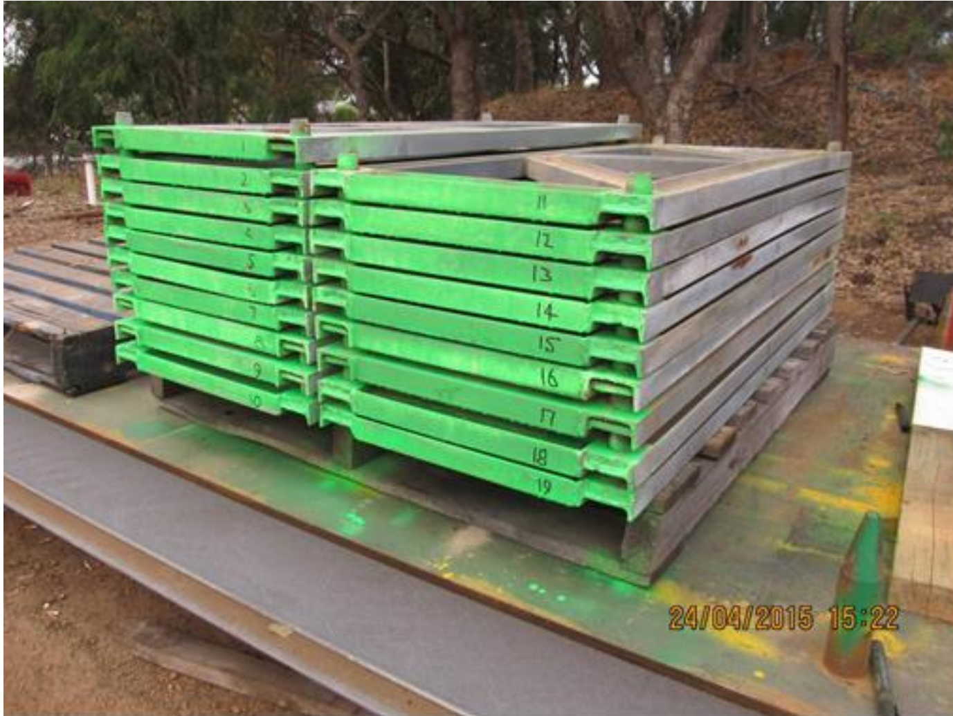
Galvanised Bracing frames in good condition
