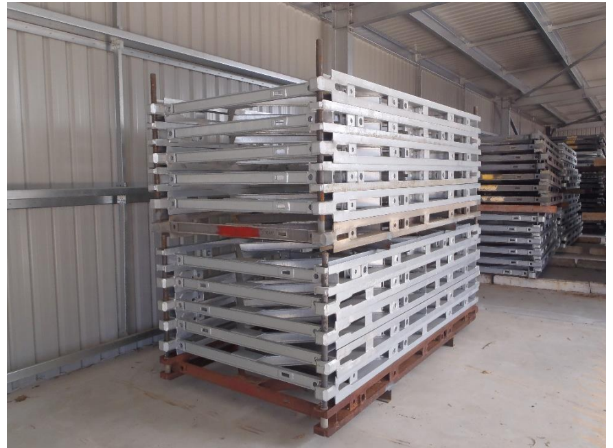
Bailey bridge panels stacked on purpose made pallets
