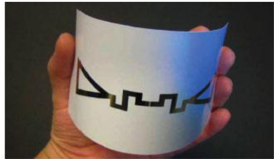
A printed, passive RFID gas sensor node on paper. The dipole antenna consists of inkjetted Ag NPs and the load in the small gap in the middle consists of inkjetted CNTs.
