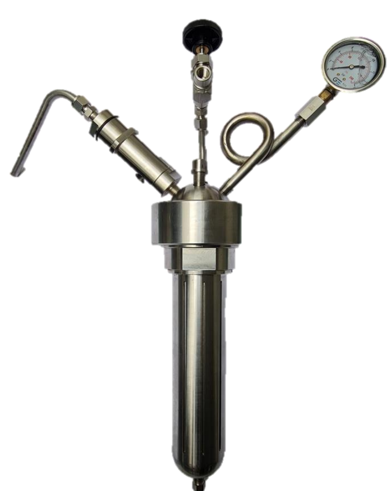
Figure.2. Picture of the 316 stainless steel carbonization reactor.
