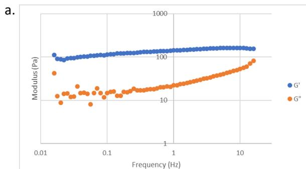
Figure 1a. Frequency sweep at a constant strain of 0.1%.
