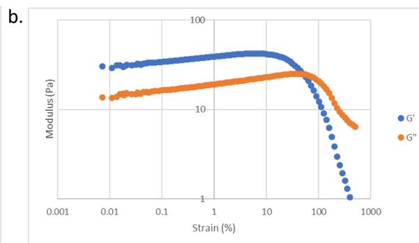
Figure 1b. Amplitude sweep at a constant frequency of 1.59 Hz.
