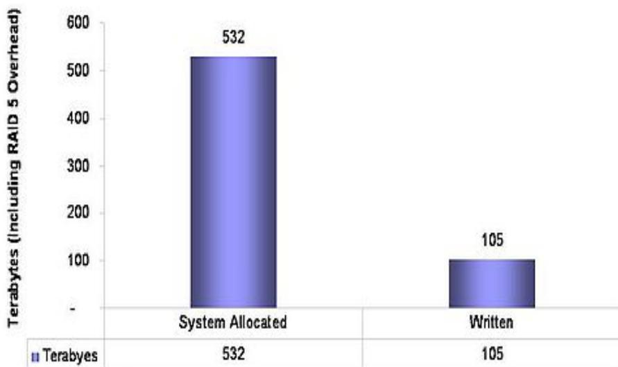
Example system “savings in storage capacity realized by thin technologies... 532 versus 105 TBs”
