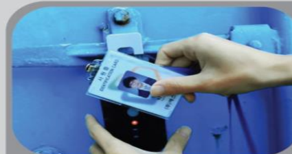
Capable of clearing seal when using certified NFC
