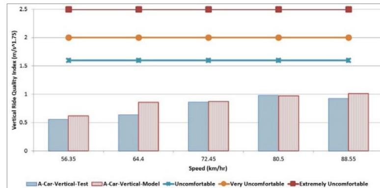
Figure 26. Ride quality – comparison of simulated vertical accelerations with test results
