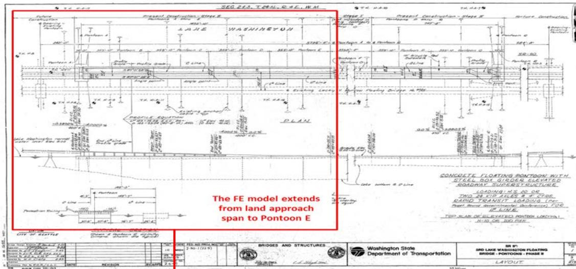
The FE model extends from land approach span to Pontoon E
