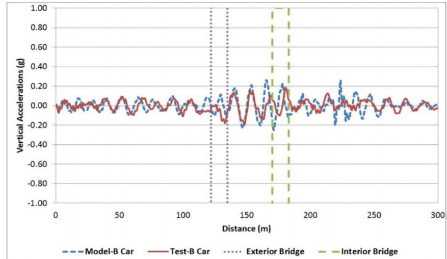
Figure 22. Vertical accelerations measured in the B-car
