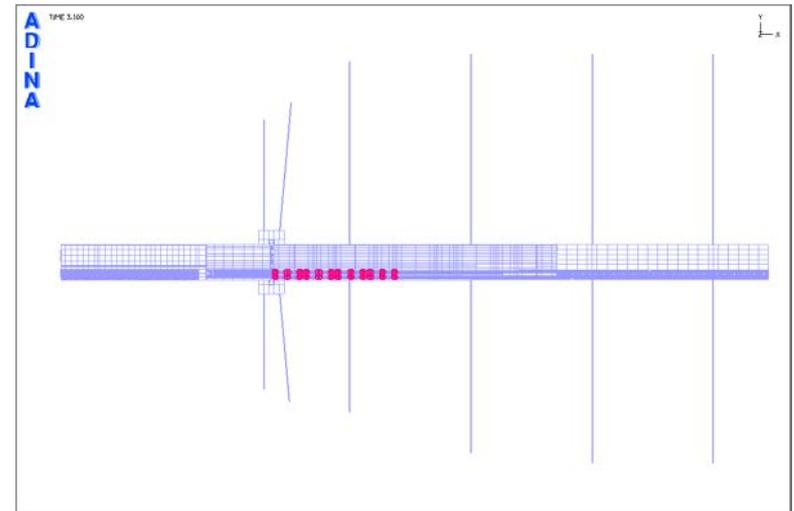
Case S7: Two sets of four trucks simulating two trains parked parallel
