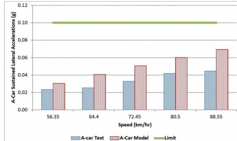
Figure 25. Ride quality – comparison of simulated lateral accelerations with test results
