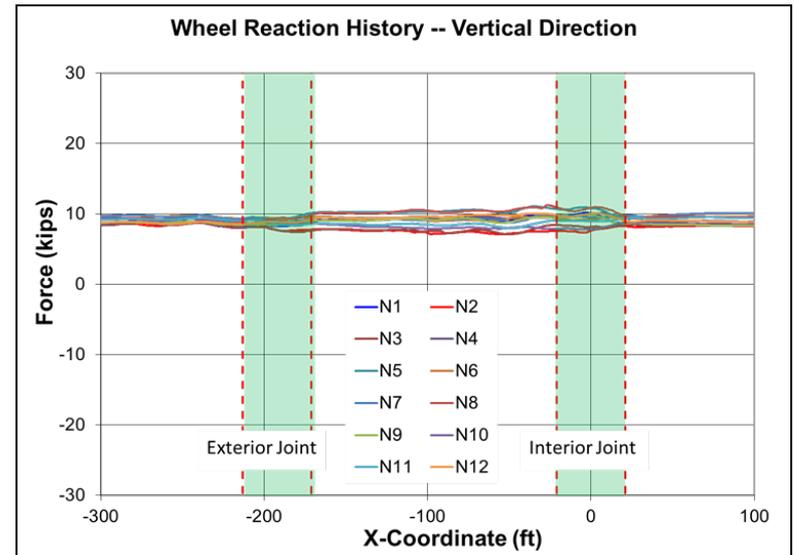
Vertical wheel reaction for Run #1 and Run #2
