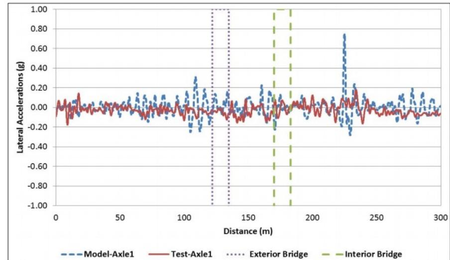
Figure 24. Lateral accelerations measured at axle 1
