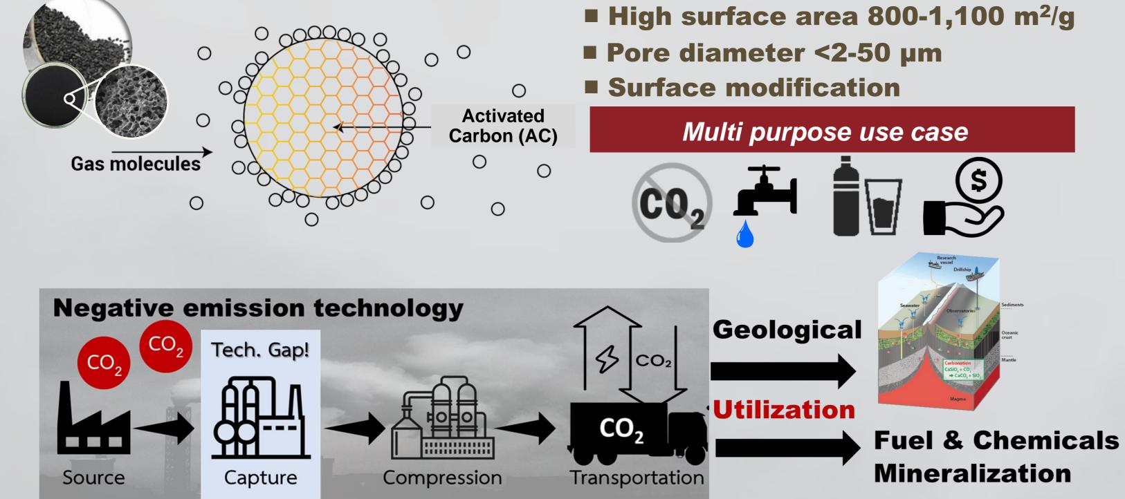
Aim: To produce micro-meso porous activated carbon from waste tire by the combination of chemical and physical methods in the fixed bed reactor for CO<sub>2</sub> adsorption.
