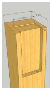
Proposed Joinery Detail: Post @ Exterior Wall (Fasteners not Shown)
