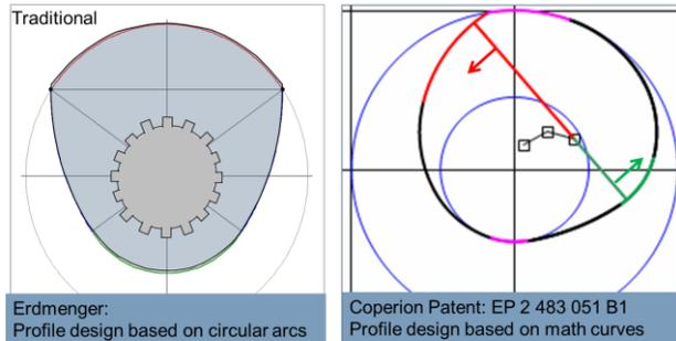
Figure 6: Traditional single flight Erdmenger design vs. and Involute single flight geometry. The Involute element is generated by the rotation of the centerline length red-green “rod” from the first contact point (far right), to the second (middle) and then the third (left)
