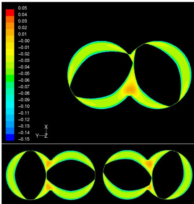
Figure 4: Simulation of axial velocity due to element rotation and material compression in the apex region.
