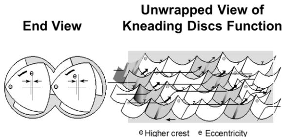
Figure 2: 3-lobe kneading block material flow.
