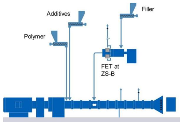
Figure 8: Process set-up for PP/PE + 70% CaCO<sub>3</sub>
