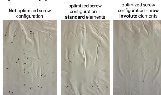
Fig.11: Filler dispersion in PE film
