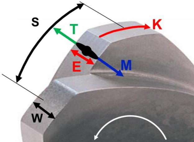
Figure 3: Kneading block key dimensions: stagger angle (W) and disc width (S). T indicates down-channel material transport, M represents back flow (distributive mixing) and E represents Extensional Flow (dispersive mixing) and K is the shear associated with any material that passes over the element crest.
