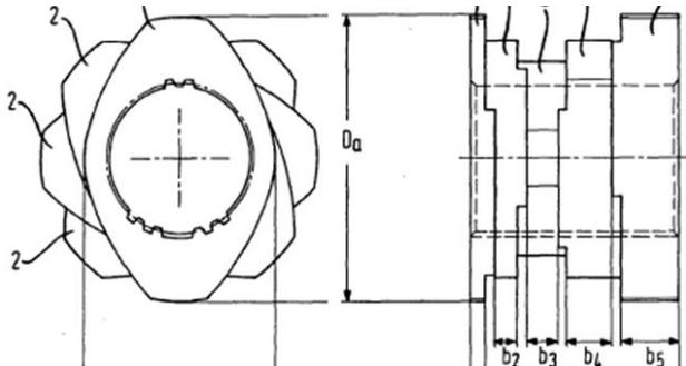
Figure 2: Progressive kneading blocks for combined distributive and dispersive mixing as described by Erdmenger
