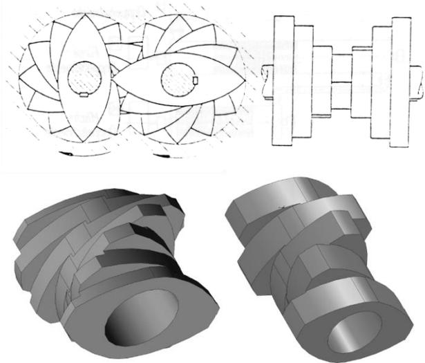
Figure 1: Comparison of original kneading block design (top) vs. the current standard kneading block (below).
