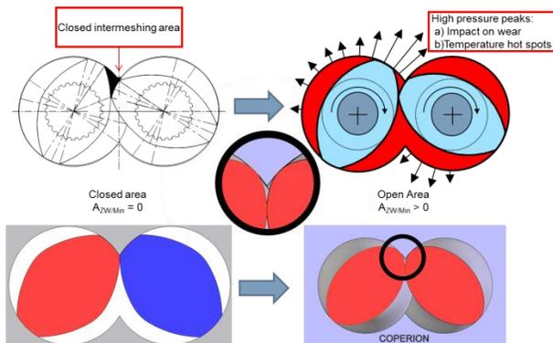
Fig. 7: Reduced pressure peaks in the APEX.
