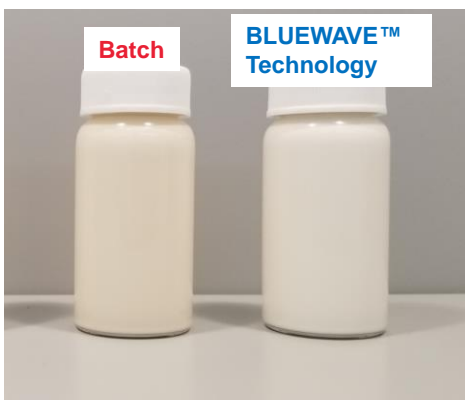
Figure 7. Appearance comparison between samples produced by means of BLUEWAVE™ Technology and batch processes.
