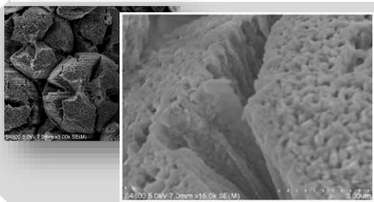
Assembly of  $MgCl_2$  nanoparticles
