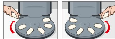
The Motion when worker taking rice ball by standing on the left side of new machine.
