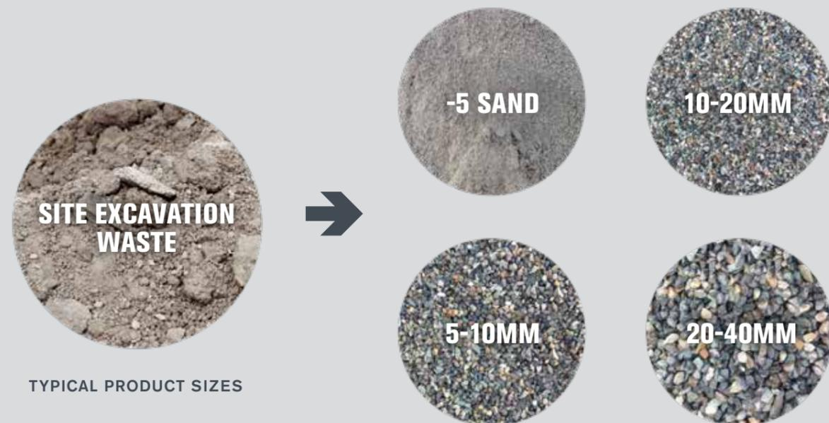
**WASHING ENABLES RECYCLABLE AGGREGATES TO FULFIL THEIR GREATEST POTENTIAL. RECYCLING TO HIGHER VALUE**
