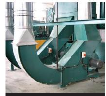
Optical sorter that separates OCC and "non-fiber" contaminants from newspaper and mixed paper grades to produce 3 outputs from 1 input.
