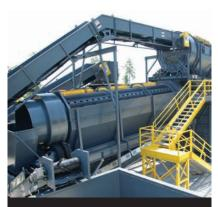
Uses a revolving screened cylinder to accomplish the separation of material by size with adjustable screening capabilities, increasing system capacity and throughput.
