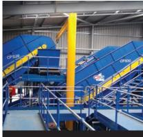
Automatically separates small fibers from containers, and 2D from 3D material with long-lasting, patented rubber cam-style discs specially engineered to resist jamming.
