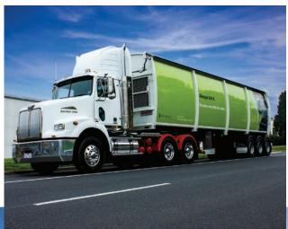
The Wastech 'Clearline' rolled wall body design provides greater durability and integral strength to withstand the high compaction forces in waste transfer station applications. The Clearline Trailer is built to withstand the high piercing forces during compaction of industrial type wastes.
