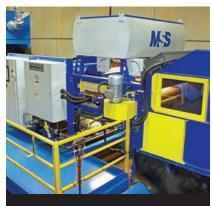
The latest in optical sorting, using new high-resolution NIR/colour sensors providing the ultimate separation performance for plastics, e-waste, and other small particle applications.
