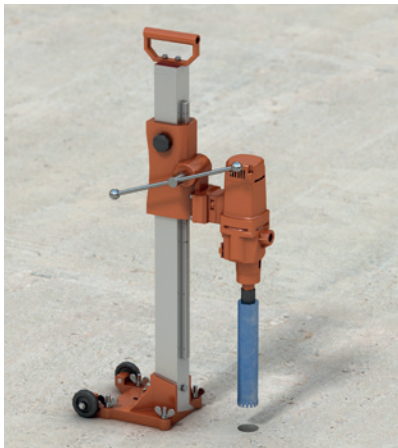
Drill concrete to specified size.
