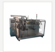
Automatically bag feeding, filling, sealing, coding and product output...
