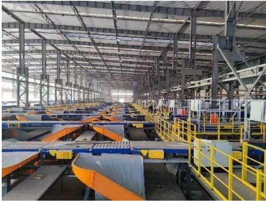
Modular belt conveyor system of China Post in Jinhua East(Zhejiang) Sorting Center
