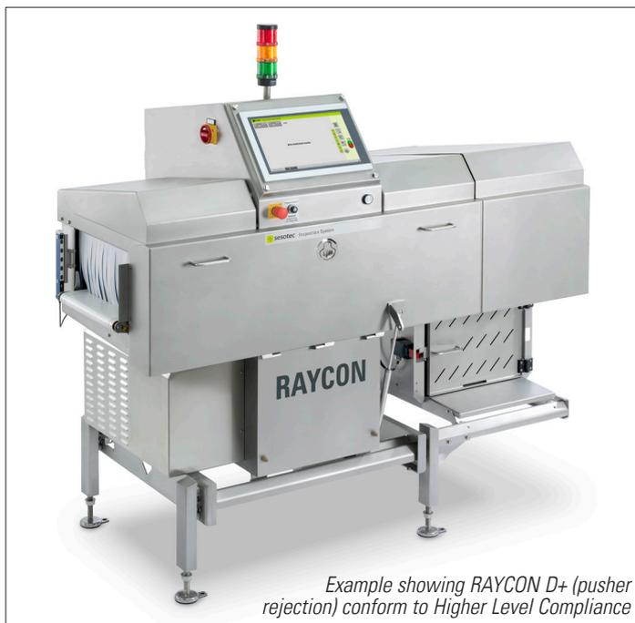
Example showing RAYCON D+ (pusher rejection) conform to Higher Level Compliance
