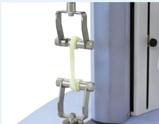
Tensile and Shearing Test for Noodles
