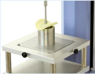
Potato Chip Breakage Test
