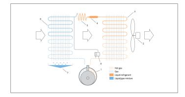
Refrigerant dehumidifiers (also known as mechanical dehumidifiers) work best in spaces where the temperature is at 20° C and above and humidity levels of 50% and above. They work on the humidity of the room and run when the humidity is above its set point.
