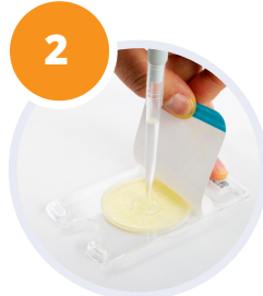
Vertically Pipet within 2 to 3 seconds
