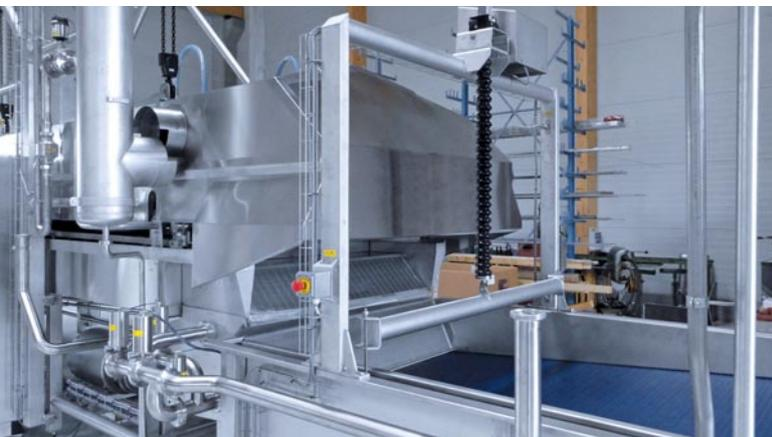
The cooling band can be lifted out for cleaning purposes using a pulley. Inductive sensors are used to detect the relevant top and bottom position.
