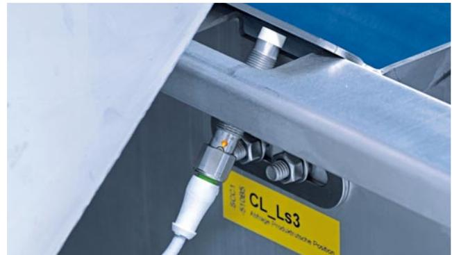
After the slot screen has been cleaned manually and returned in place, production can only be resumed after it has been released by the inductive sensor.
