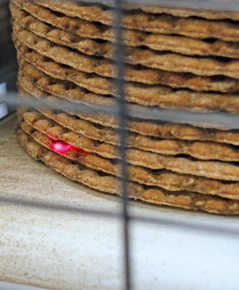
under severe conditions and ensures an extremely long life time. The O6 sensors are now also available as versions with IO-Link. Via this interface, the range, sensitivity, light-on / dark-on modes, switching delay or deactivation of the operating elements can, for example, be set remotely.
