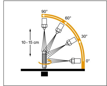
**IP 69K high-pressure cleaning test**
