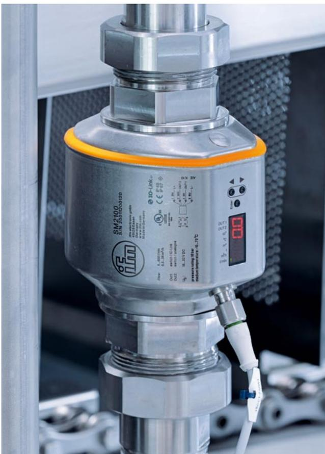
*The magmeter SM2100 is used to detect the current flow velocity as well as the total quantity of the feed water supply. Both values are transferred using IO-Link to the control system.*
