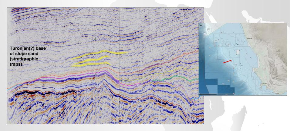
blue: positive reflection coefficient brown: negative reflection coefficient
