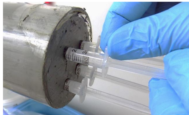
Head space gas samples are taken after core recovery.
