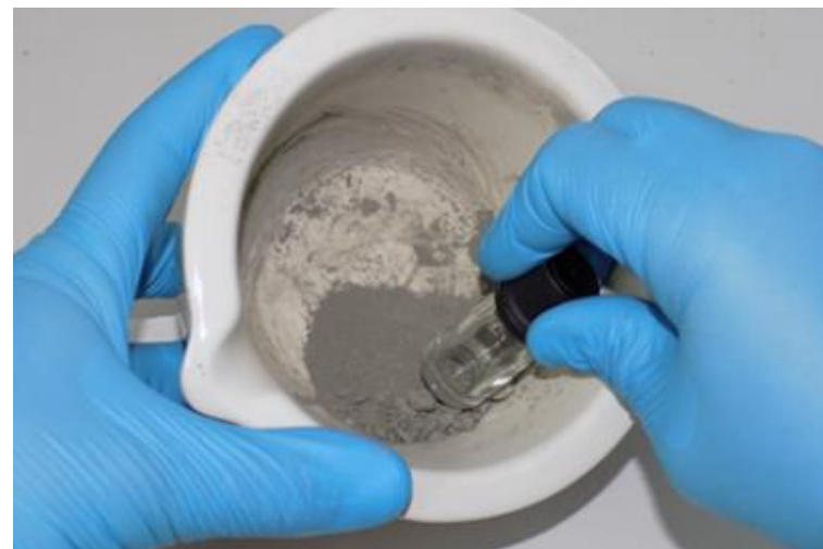
Samples for TSF analysis are dried, powdered, and extracted.
