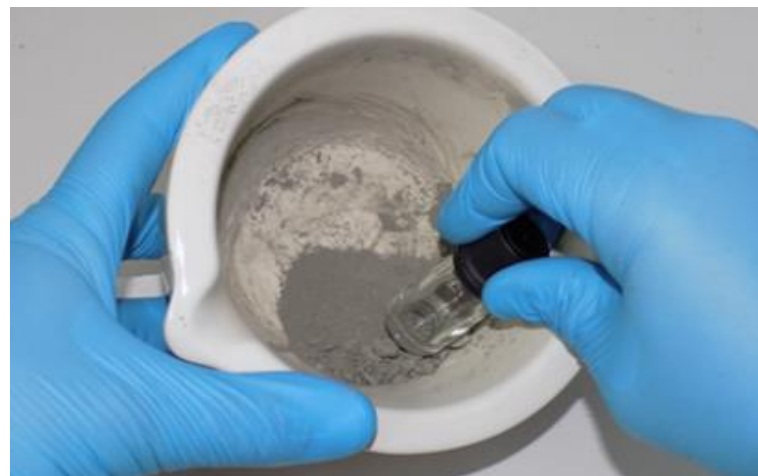
Samples for TSF analysis are dried, powdered, and extracted.
